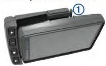
2 Tilt your device back until it snaps into place and the top of the latch is flush with the surrounding surface of the motorcycle mount.
