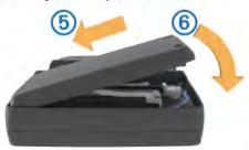
8 Close the battery cover 6 and tighten the screws.
