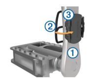
4 Rotate the crank arm to check for clearance. The sensor and bands should not contact any part of your bike or shoe.
