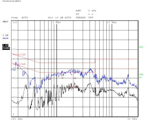
Figure 9 AC Line Conducted emissions of EUT line 1 (EUT-USB-CPU AC Adapter)
