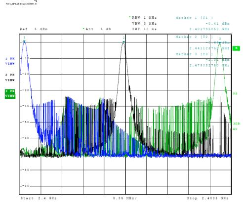
Figure 11 Plot of Transmitter Emissions (In 2402-2479 MHz Band, Mode 1)
