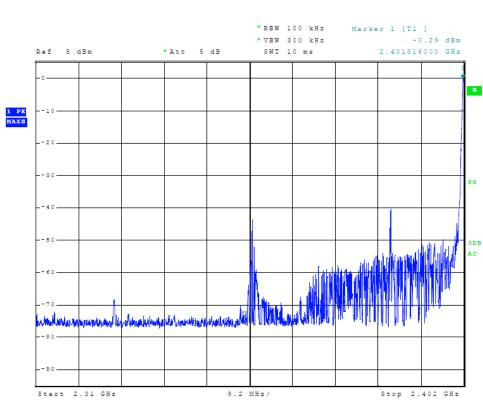
Figure 13 Plot of Transmitter Emissions (Low Band Edge, Mode 1)
