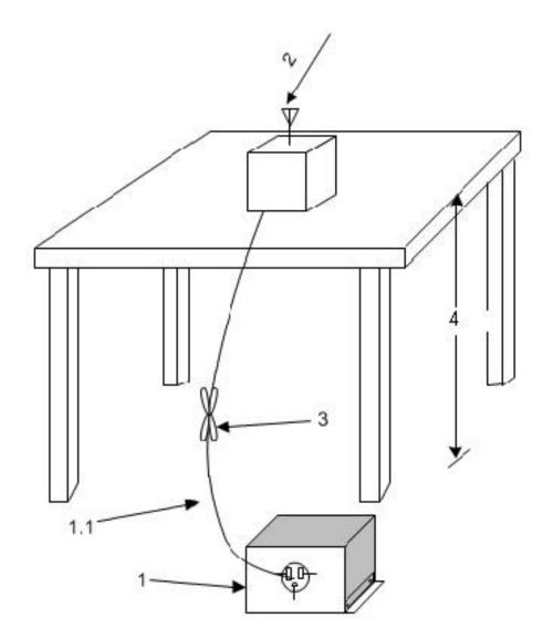
1—A LISN is optional for radiated measurements between 30 MHz and 1000 MHz but not allowed for measurements below 30 MHz and above 1000 MHz (see 6.3.1). If used, then connect EUT to one LISN. Unused LISN measuring port connectors shall be terminated in 50  $\Omega$  loads. The LISN may be placed on top of, or immediately beneath, the reference ground plane (see 6.2.2 and 6.2.3.2).
