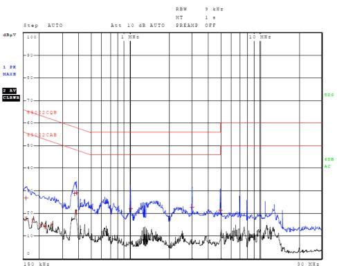
Figure 4 AC Line Conducted emissions of EUT line 2 (EUT AC Adapter 326-00072-00)
