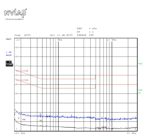
Figure 7 AC Line Conducted emissions of EUT line 1 (EUT AC Adapter 326-00087-00)
