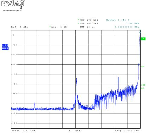
Figure 17 Plot of Transmitter Emissions (Low Band Edge, Mode 2)
