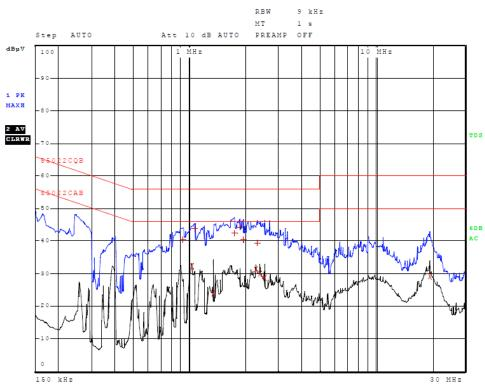
Figure 10 AC Line Conducted emissions of EUT line 2 (EUT-USB-CPU AC Adapter)
