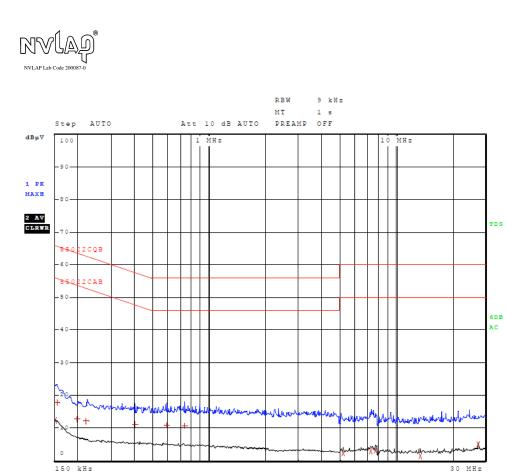
Figure 5 AC Line Conducted emissions of EUT line 1 (EUT AC Adapter 326-00086-01)
