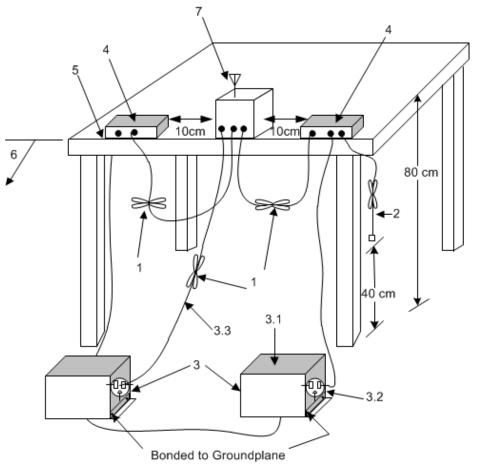
1—Interconnecting cables that hang closer than 40 cm to the ground plane shall be folded back and forth in the center forming a bundle 30 cm to 40 cm long see (see 6.2.3.2).
