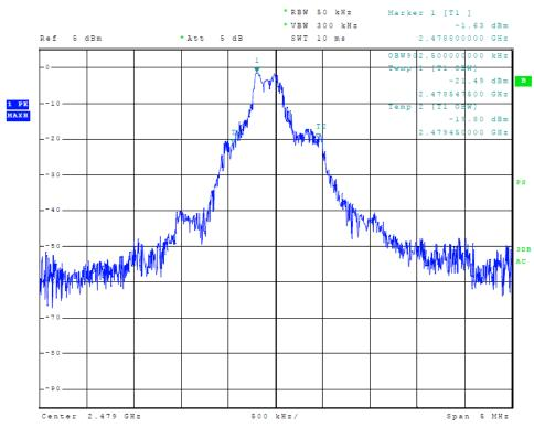
Figure 12 Plot of Transmitter Emissions (2402-2479 MHz, 99% Occupied Bandwidth, Mode 1)
