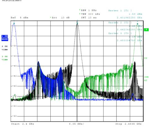
Figure 15 Plot of Transmitter Emissions (In 2402-2480 MHz Band, Mode 2)
