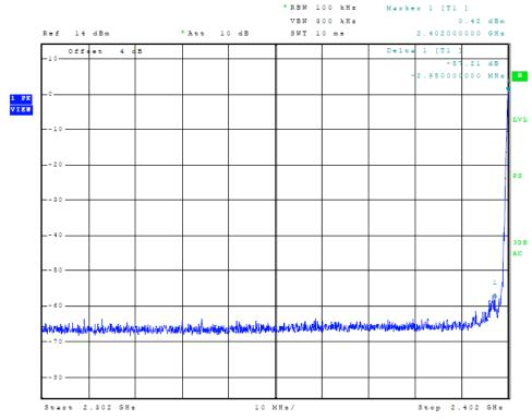
Figure 9 Plot of Transmitter Emissions (GFSK, Low Band Edge)
