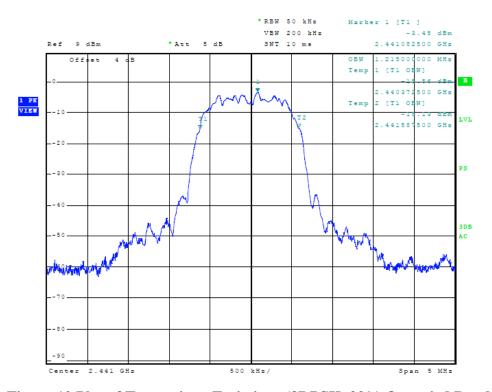
Figure 12 Plot of Transmitter Emissions (8DPSK, 99% Occupied Bandwidth)
