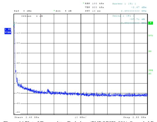
Figure 16 Plot of Transmitter Emissions (Pi4DQPSK, 99% Occupied Bandwidth)
