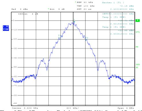
Figure 8 Plot of Transmitter Emissions (GFSK, 99% Occupied Bandwidth)
