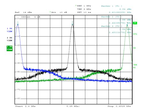
Figure 11 Plot of Transmitter Emissions (8DPSK Operation in 2402-2480 MHz)
