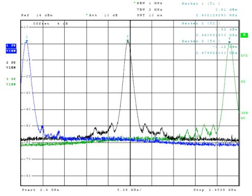
Figure 7 Plot of Transmitter Emissions (GFSK, Operation in 2402-2480 MHz)
