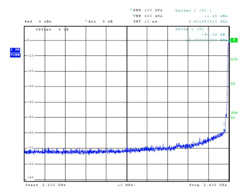
Figure 13 Plot of Transmitter Emissions (8DPSK, Low Band Edge)
