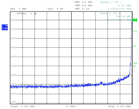
Figure 17 Plot of Transmitter Emissions (Pi4DQPSK, Low Band Edge)
