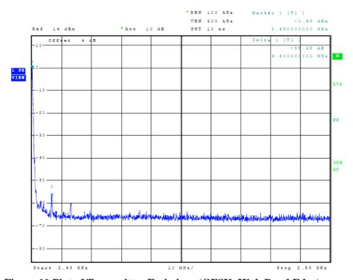
Figure 10 Plot of Transmitter Emissions (GFSK, High Band Edge)
