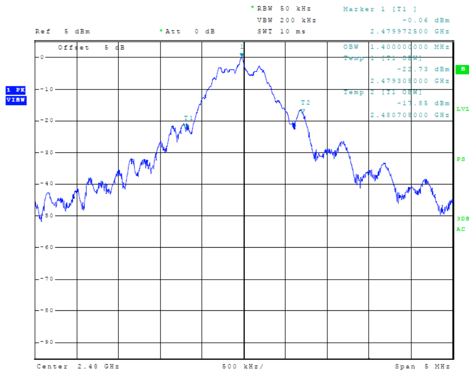
Figure 2 Plot of Transmitter Emissions (2402-2480 MHz, 99% Occupied Bandwidth)
