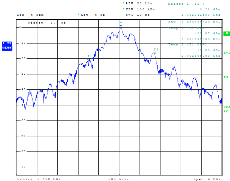
Figure 16 Plot of Transmitter Emissions (99% Occupied Bandwidth) (Mode 2)
