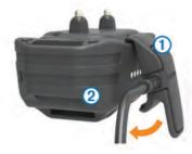
2 Plug the power cable into a power source.
