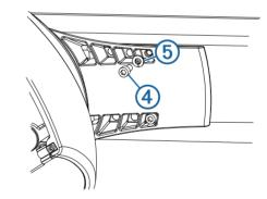
4 Torque the hex bolts to 0.81 kgf-m (70 lfb-in. [6 lbf-ft.]) to fasten the antenna to the pedestal without damaging the antenna or the mounting hardware.
