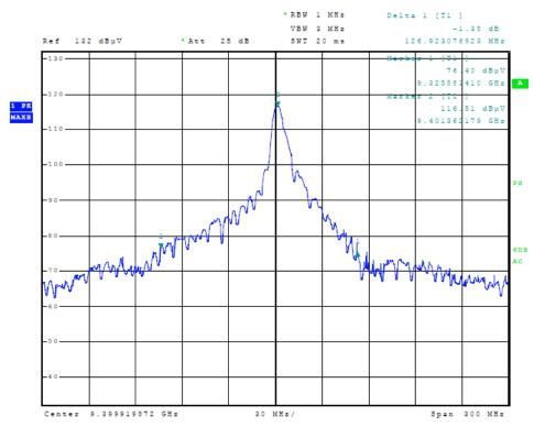
Figure 3 Plot of analyzer screen showing 40-dB occupied bandwidth (1/2 nm)
