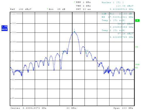
Figure 2 Plot of analyzer screen showing 23-dB occupied bandwidth (1/2 nm)
