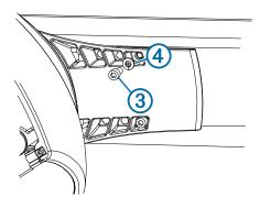
**4** Torque the hex bolts to 0.81 kgf-m (70 lfb-in. [6 lbf-ft.]) to fasten the antenna to the unit base without damaging the antenna or the mounting hardware.
