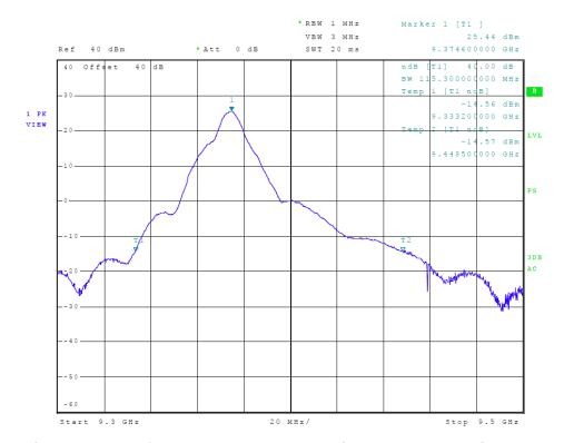
Figure 3 Plot of analyzer screen showing 40-dB occupied bandwidth
