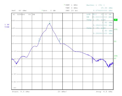
Figure 2 Plot of analyzer screen showing 23-dB occupied bandwidth
