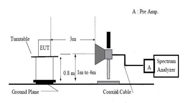
(C) Substituted Method Test setup:
