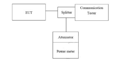
Measurement Setup for testing on Antenna connector.
