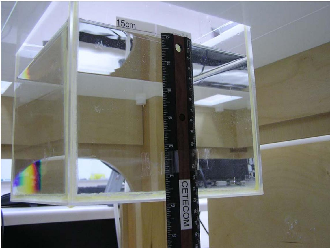
**Photo 2. Photo to demonstrate 15 cm Z-axis flat phantom**
