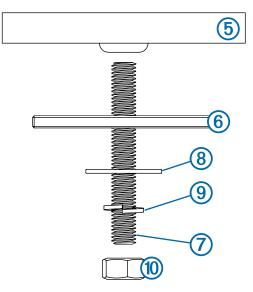
**10** Using a torque wrench, tighten the nuts from 13.7 to 18.6 Nm (10 to 14 lbf-in.) of force.
