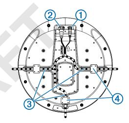
4 Press the cables into any of the guide grooves ③ on the bottom of the case, and secure them using cable hold-down plates ④.
