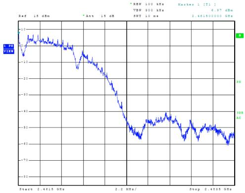
Figure 5 Plot of High Band Edge (802.11 B-Mode)
