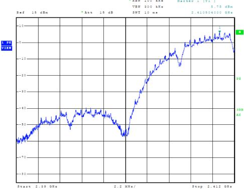
Figure 4 Plot of Low Band Edge (802.11 B-Mode)
