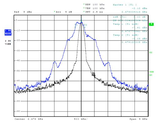
Figure Thirteen Occupied Bandwidth (high channel)
