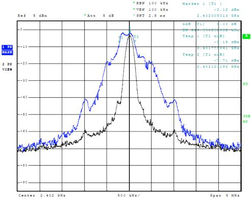
Figure Eleven Occupied Bandwidth (low channel)
