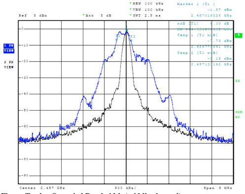
Figure Twelve Occupied Bandwidth (middle channel)
