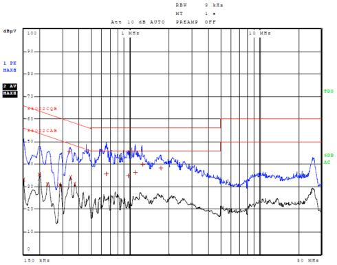
Figure One AC Line Conducted emissions of EUT line 1 (EUT AC Adapter, 362-00054-01)
