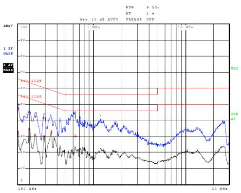
Figure Two AC Line Conducted emissions of EUT line 2 (EUT AC Adapter, 362-00054-01)
