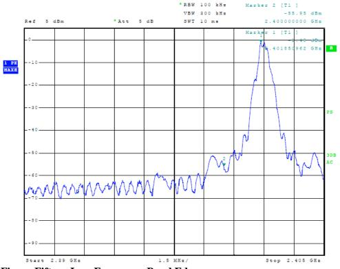
**Figure Fifteen Low Frequency Band Edge**
