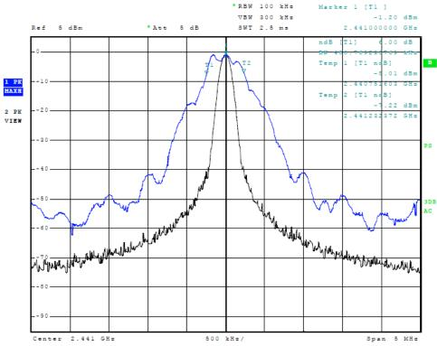
Figure Twelve Occupied Bandwidth (middle channel)
