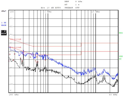
Figure Three AC Line Conducted emissions line 1 (EUT/CPU)
