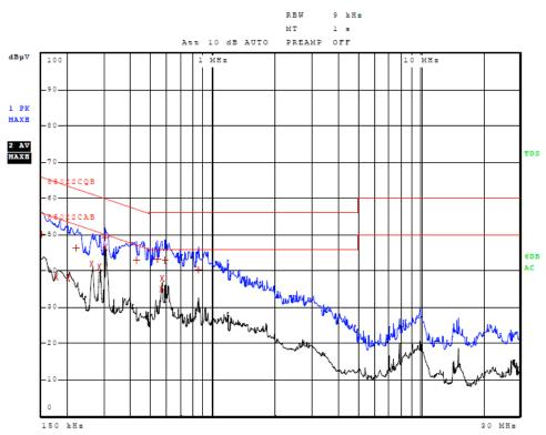
Figure Four AC Line Conducted emissions line 2 (EUT/CPU)
