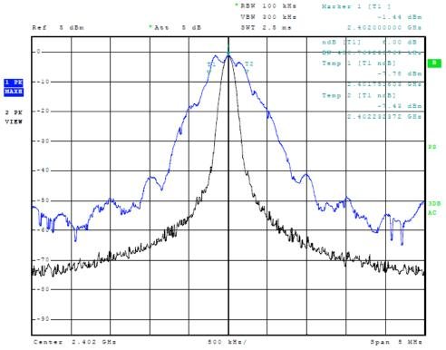
Figure Eleven Occupied Bandwidth (low channel)
