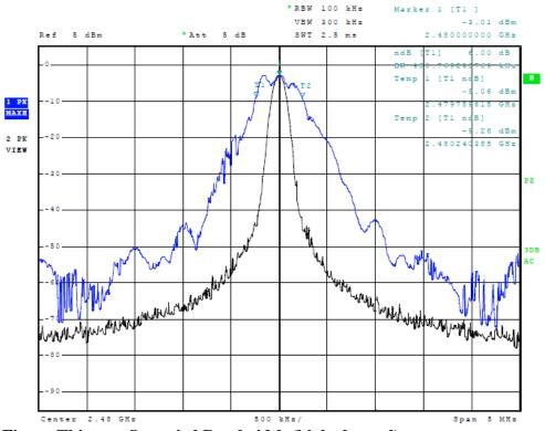
Figure Thirteen Occupied Bandwidth (high channel)
