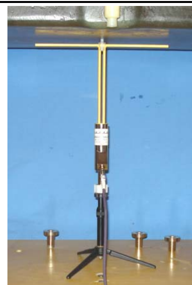
SPEAG 450 MHz Validation Dipole Setup
