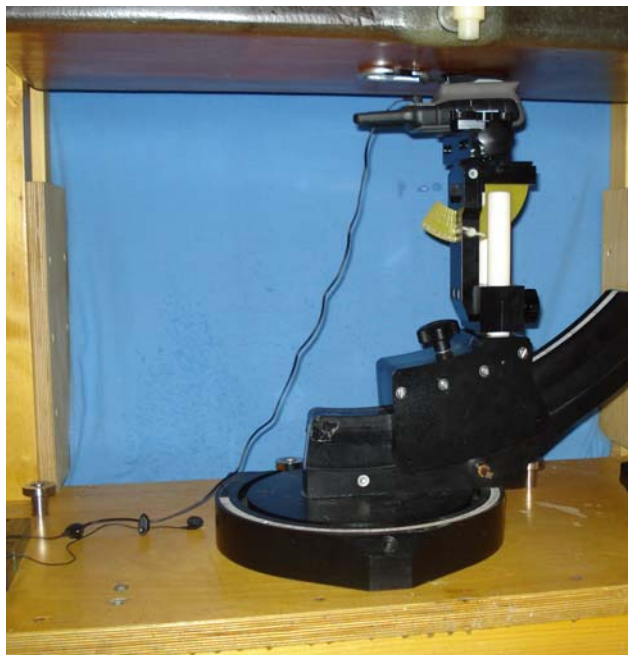
Body-worn Configuration – DUT with Alkaline Battery, Carabiner Clip and Earbud w/ PTT
