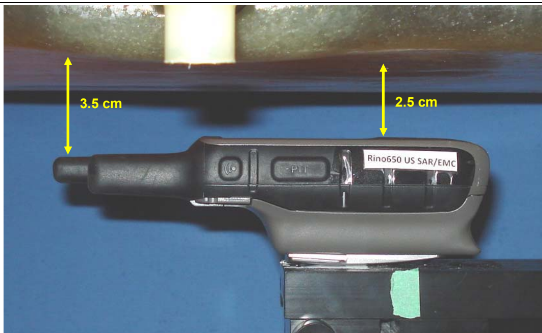
Face-held Configuration – 2.5 cm spacing from front keypad side of radio to planar phantom – DUT with Alkaline battery pack
