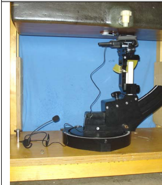
Body-worn Configuration – DUT with Alkaline Battery Pack, Carabiner Clip and Headset-Mic - separation distances same as Page 87
