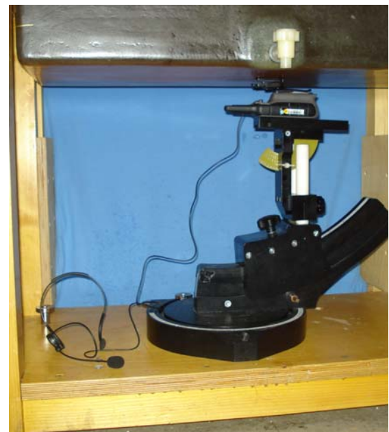
Body-worn Configuration – DUT with Alkaline Battery Pack, Belt-Clip and Headset-Mic - separation distances same as listed on Page 84
