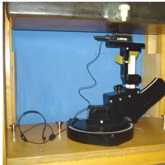
Body-worn Configuration – DUT with Li-ion Battery Pack, Belt-Clip and Headset-Mic - separation distances same as listed on Page 84
