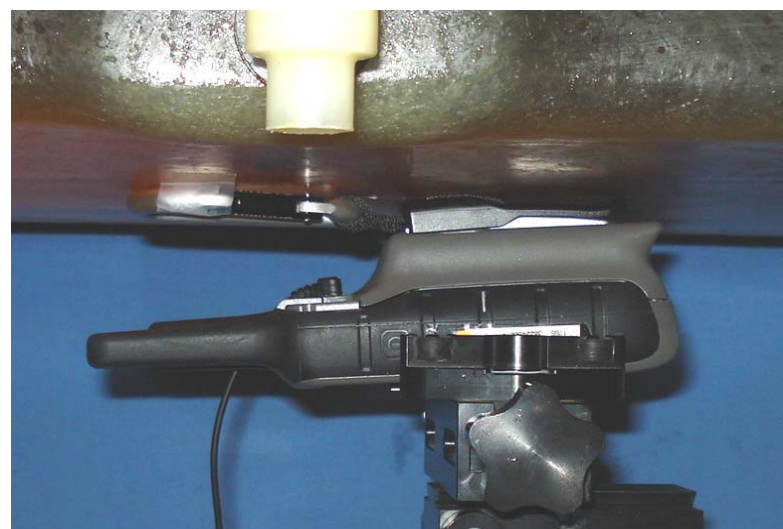
Body-worn Configuration – DUT with Alkaline Battery Pack, Carabiner Clip and Headset-Mic - separation distances same as Page 87
