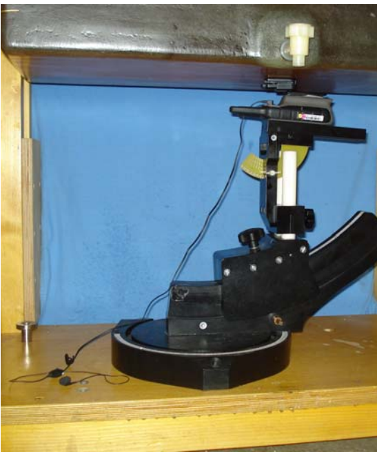
Body-worn Configuration – DUT with Alkaline Battery Pack, Belt-Clip and Earbud w/ PTT
