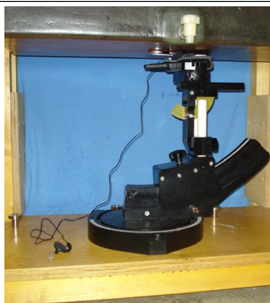
Body-worn Configuration – DUT with Li-ion Battery Pack, Carabiner Clip and Ear Receiver - separation distances same as Page 87
