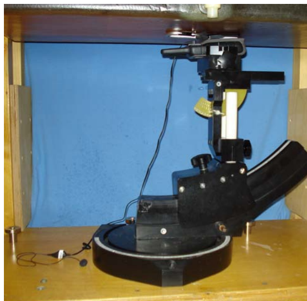
Body-worn Configuration – DUT with Li-ion Battery, Carabiner Clip and Earbud w/ PTT
