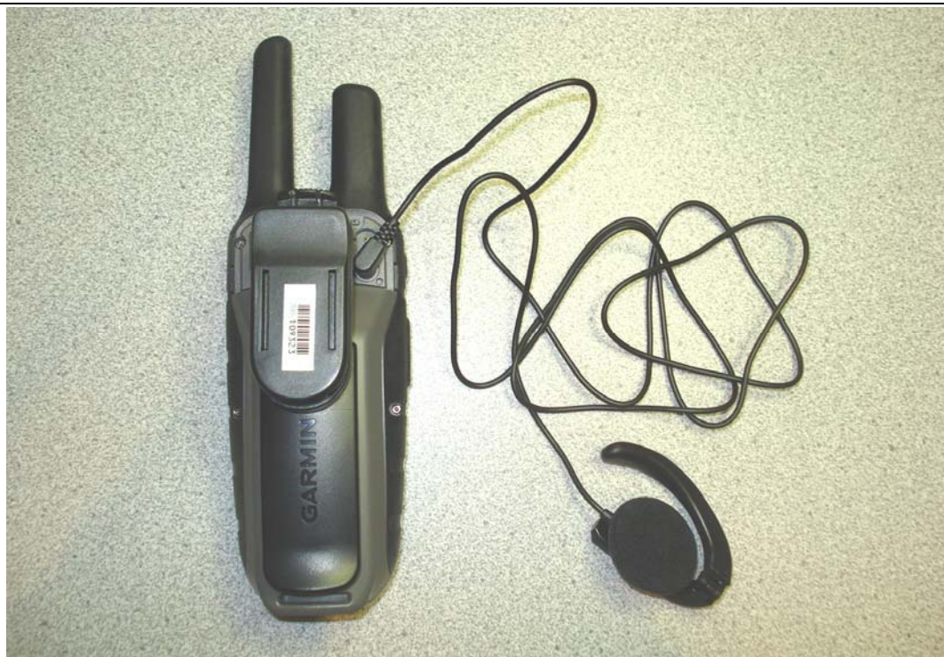
Back of DUT with Lithium Ion battery, Belt-Clip accessory, and Ear Receiver audio accessory
