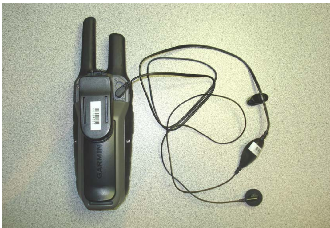
Back of DUT with Lithium Ion battery, Belt-Clip accessory, and Earbud w/ PTT audio accessory
