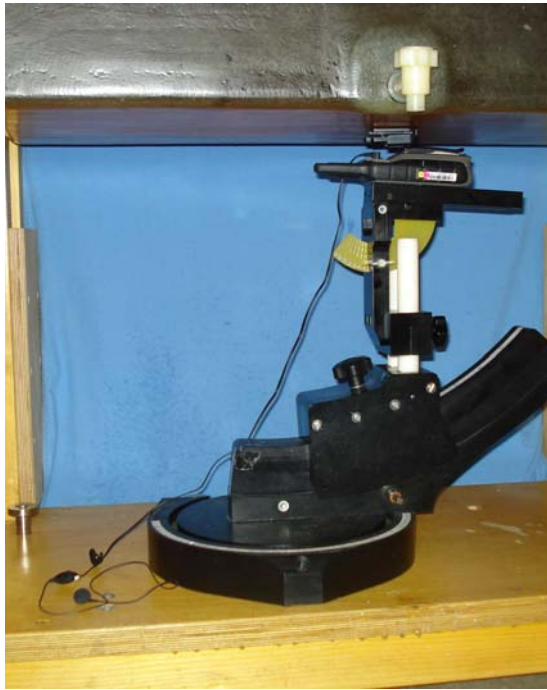
Body-worn Configuration – DUT with Li-ion Battery Pack, Belt-Clip and Earbud w/ PTT
