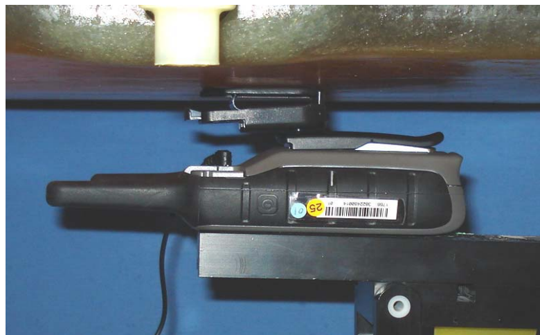
Body-worn Configuration – DUT with Li-ion Battery Pack, Belt-Clip and Headset-Mic - separation distances same as listed on Page 84
