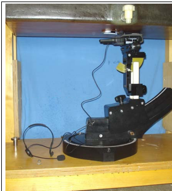
Body-worn Configuration – DUT with Li-ion Battery Pack, Carabiner Clip and Headset-Mic - separation distances same as Page 87
