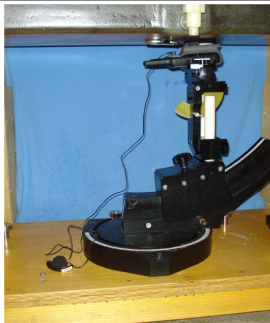
Body-worn Configuration – DUT with Alkaline Battery Pack, Carabiner Clip and Ear Receiver - separation distances same as Page 87
