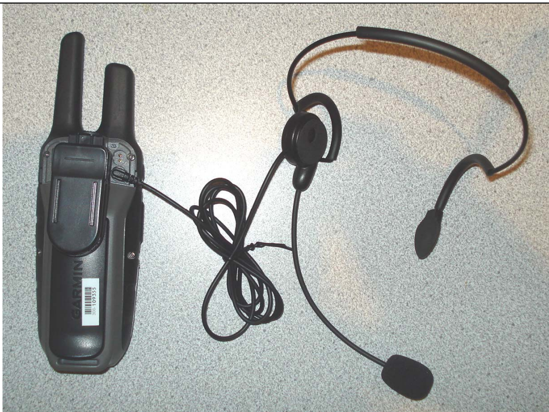
Back of DUT with Lithium Ion battery, Belt-Clip accessory, and Headset audio accessory
