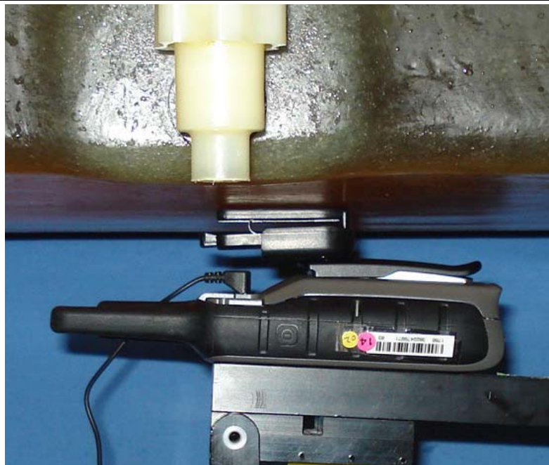
Body-worn Configuration – DUT with Li-ion Battery Pack, Belt-Clip and Ear Receiver - separation distances same as listed on Page 84
