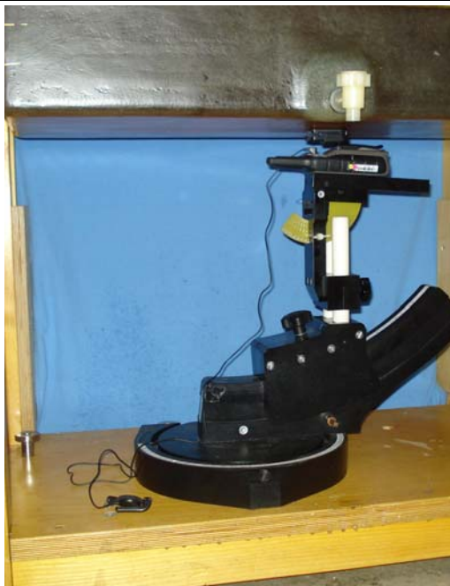
Body-worn Configuration – DUT with Li-ion Battery Pack, Belt-Clip and Ear Receiver - separation distances same as listed on Page 84
