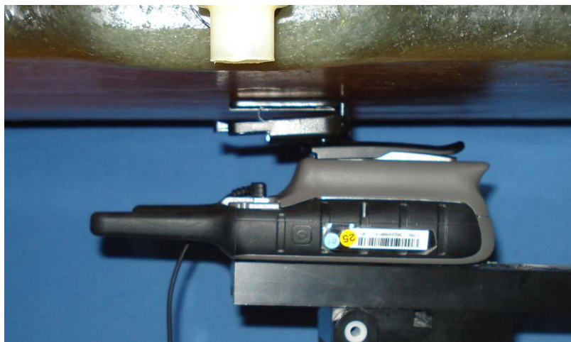
Body-worn Configuration – DUT with Alkaline Battery Pack, Belt-Clip and Headset-Mic - separation distances same as listed on Page 84
