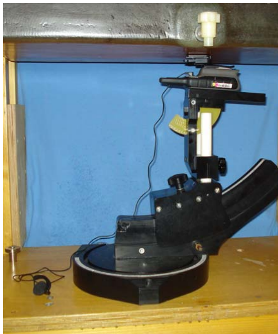
Body-worn Configuration – DUT with Alkaline Battery Pack, Belt-Clip and Ear Receiver - separation distances same as listed on Page 84
