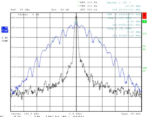
Figure 3 Occupied Band Width (Data 0101)
