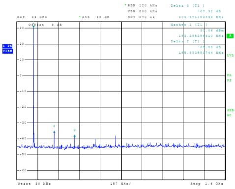
Figure 6 Spurious Emissions at Antenna Terminal
