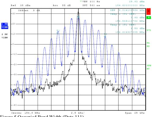
Figure 5 Occupied Band Width (Data 111)
