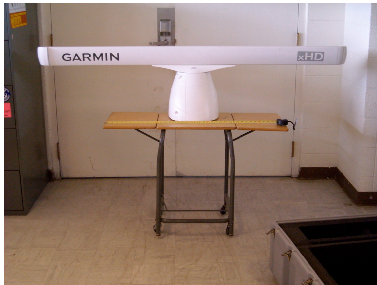
Figure 9. Exterior of the EUT. The radiating element is approximately 2 meters between endpoints.
