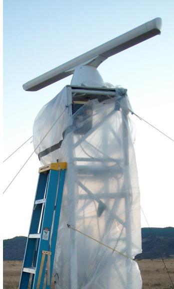
Figure 8. EUT mounted on the test platform. The pedestal was enclosed in plastic to protect the power supply.
