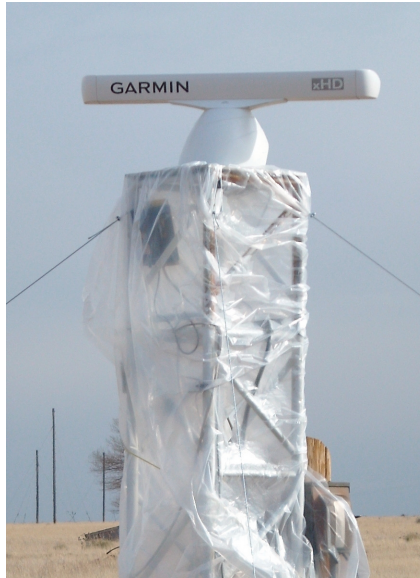
Figure 8. EUT mounted on the test platform. The pedestal was enclosed in plastic to protect the power supply.
