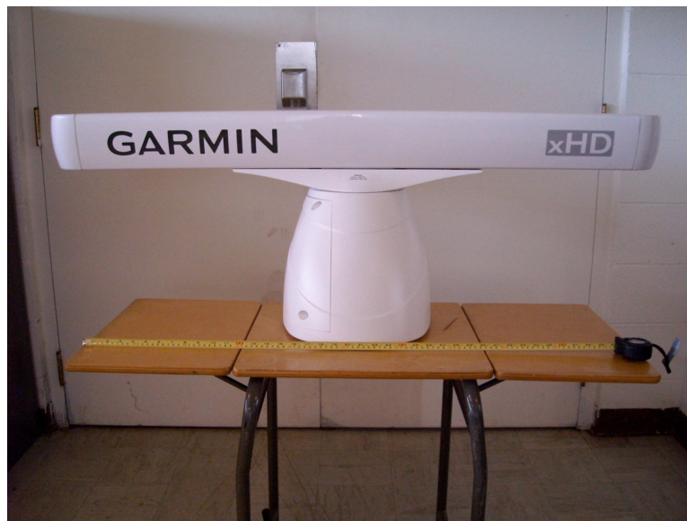
Figure 9. Exterior of the EUT. The radiating element is approximately 1 meter between endpoints.
