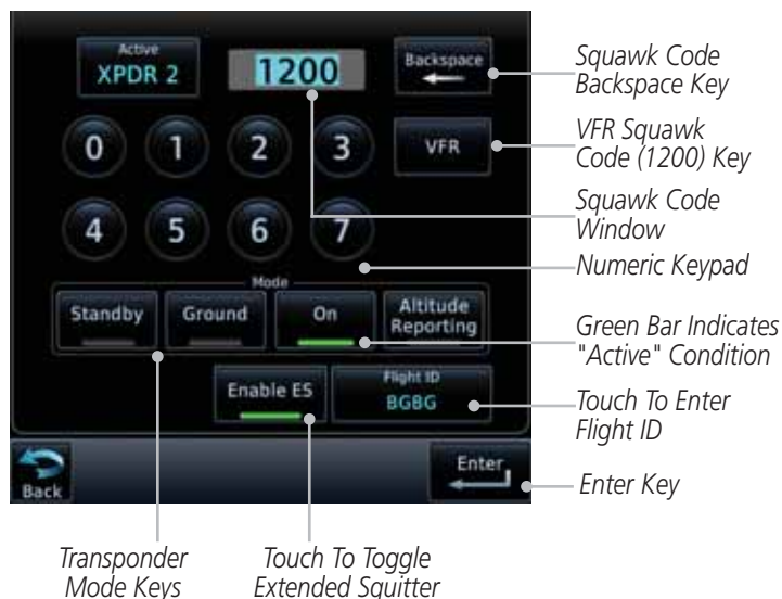
Figure 2-12 Transponder Control Panel With Extended Squitter Capability
