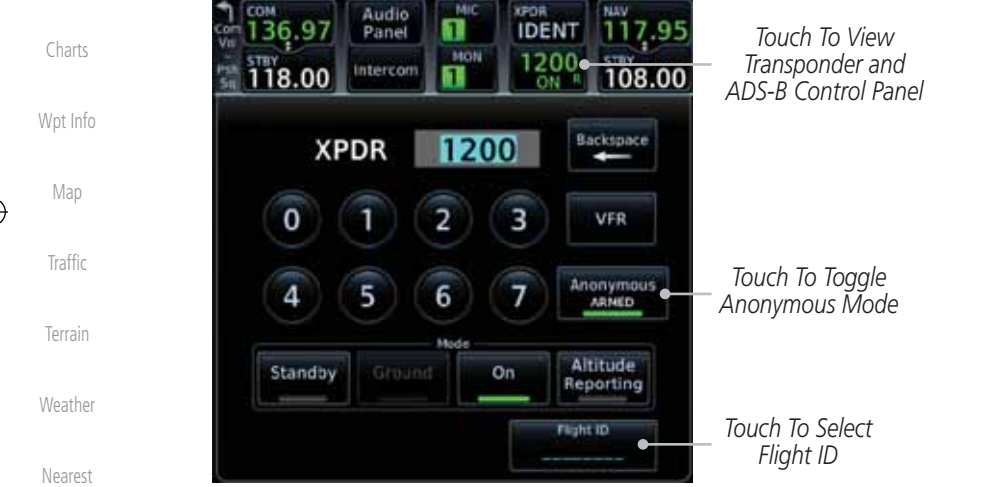
Figure 2-11 ADS-B/Transponder Control Panel
