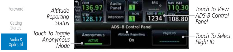
Figure 2-10 ADS-B Control Panel
