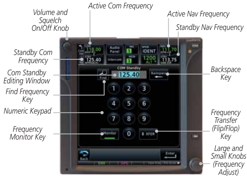
Figure 3-1 Nav/Com Controls
