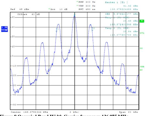
Figure 8 Occupied Band Width Carrier frequency 136.975 MHz
