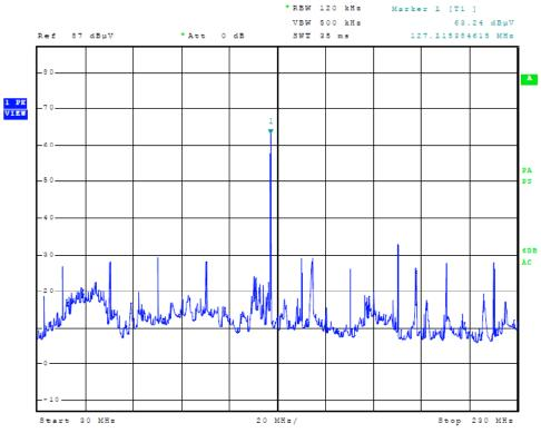
Figure 10 Radiated emissions taken at 1 meter in screen room
