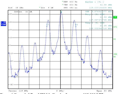
Figure 6 Occupied Band Width Carrier frequency 118.000 MHz
