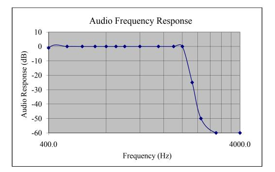
Figure 5 shows the frequency response of the audio low pass filter.
