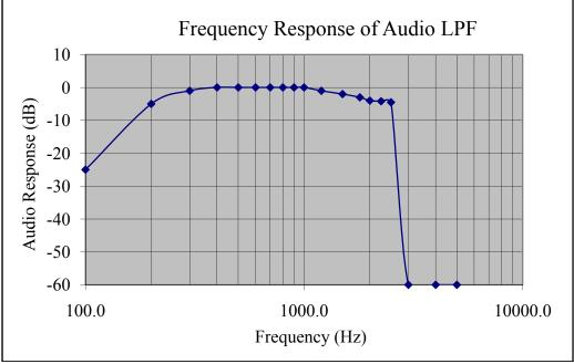
Figure 5 Frequency Response of Audio Low pass Filter
