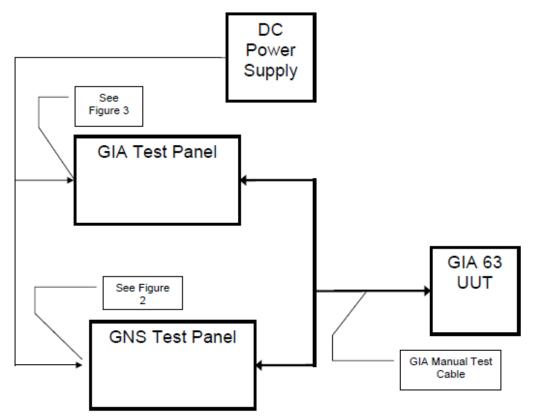
Figure 1: Test Setup Block Diagram
