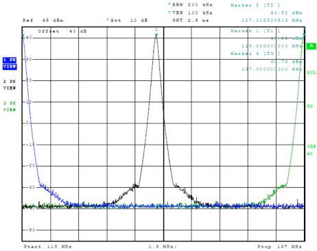
Figure 2 Maximum Power Output (14 Volt Input)
