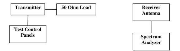
The test setup was assembled in a screen room for preliminary screening. The transmitter was placed on a wooden turntable 0.8 meters above the ground plane and at a distance of 1 meter from the receive antenna, plots were taken of the radiated emissions. Refer to figures 10 and 11 showing plots of the spectrum analyzer display of the radiated emissions frequency spectrum taken in the screen room.
