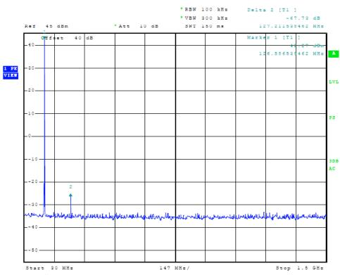
Figure 9 Spurious Emissions at Antenna Terminal
