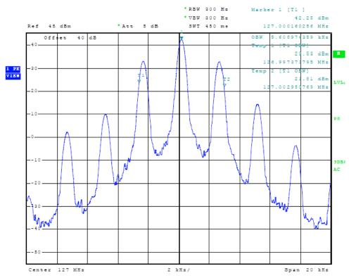
Figure 7 Occupied Band Width Carrier frequency 127.000 MHz
