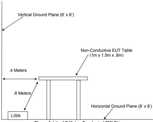
Figure 2.4-1: AC Mains Conducted EMI Site
