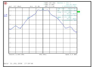
Figure 7.4-1: 20dB Bandwidth Low Channel
