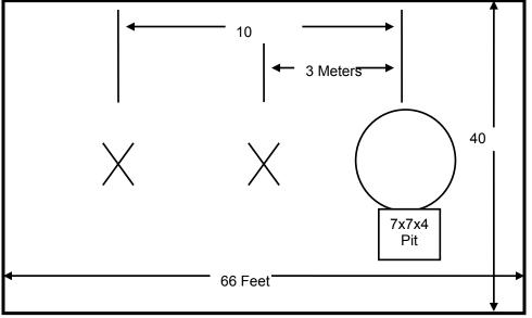
A diagram of the Open Area Test Site is shown in Figure 2.3-2 below:
