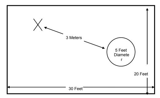
A diagram of the Semi-Anechoic Chamber Test Site is shown in Figure 2.3-1 below:
