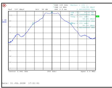
Figure 7.4-2: 20dB Bandwidth Mid Channel
