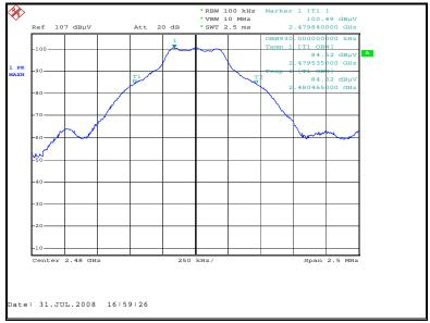
Figure 7.4-6: 99% Bandwidth High Channel
