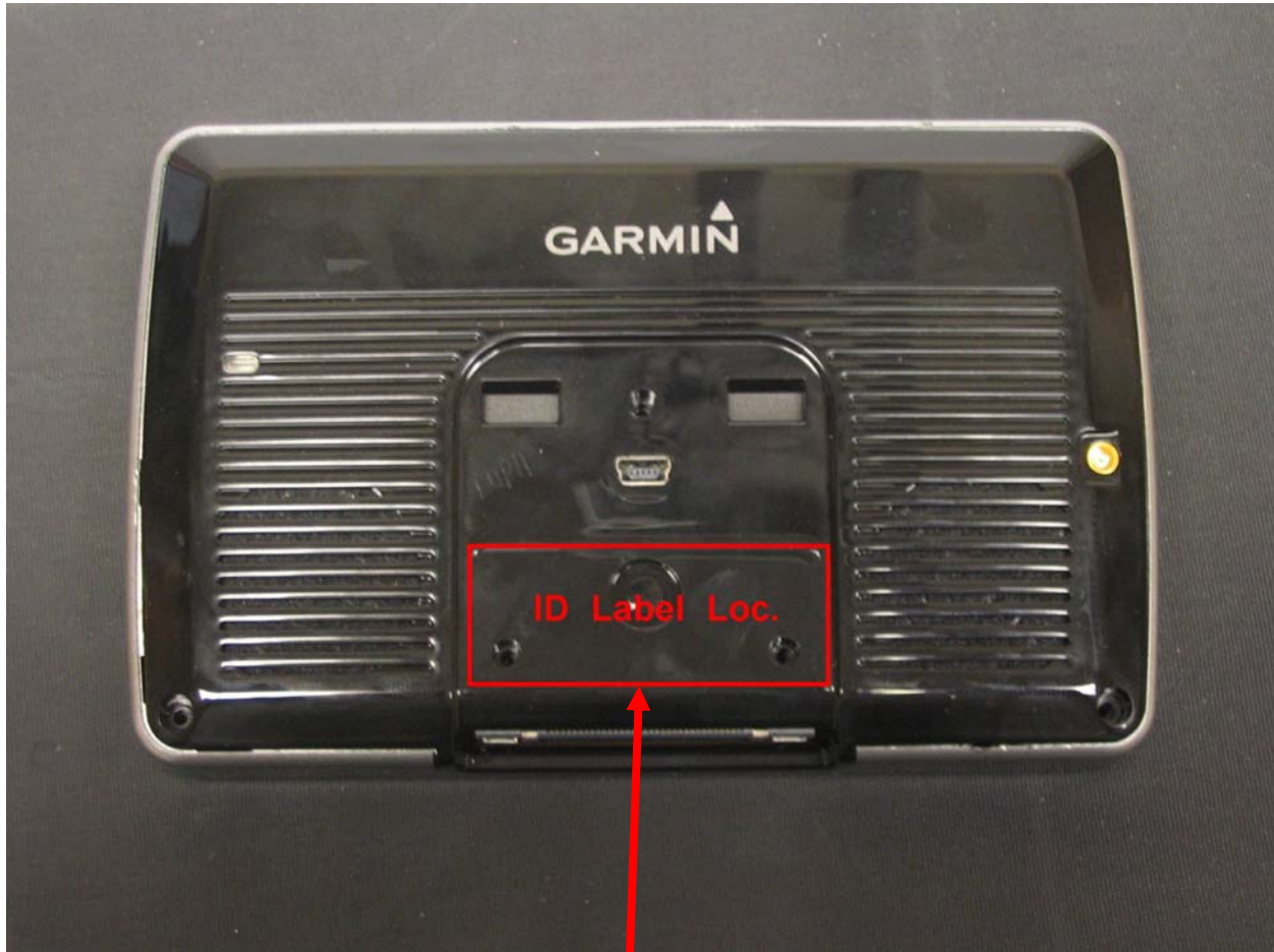
Photograph of equipment Label Placement and drawing of label
