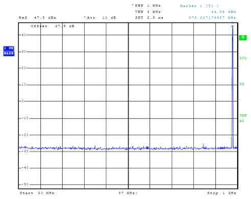
Figure 6 Spurious Emissions at Antenna Terminal (UAT 978 MHz T1)
