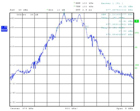
Figure 4 Occupied Band Width, Carrier frequency 978.00 MHz
