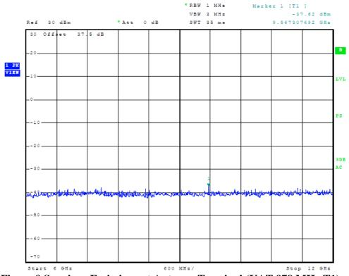
Figure 9 Spurious Emissions at Antenna Terminal (UAT 978 MHz T1)
