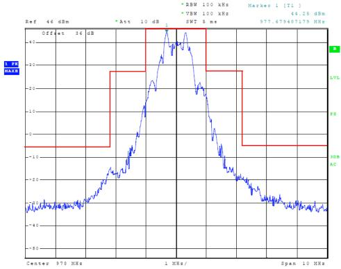
Figure 10 Emissions Mask (UAT 978 MHz)
