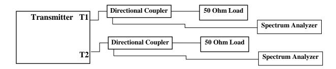
A Rohde & Schwarz ESU 40 spectrum analyzer was used to observe the radio frequency spectrum with the transmitter operating in all normal modes. The EUT was set to transmit in typical mode while measurements were made.
