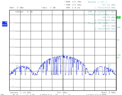
Figure 5 Occupied Band Width, Carrier frequency 1030.00 MHz
