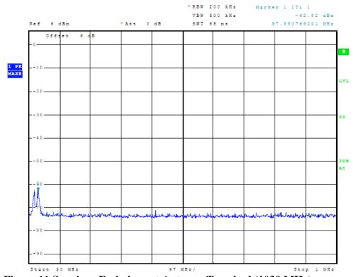
Figure 11 Spurious Emissions at Antenna Terminal (1030 MHz)
