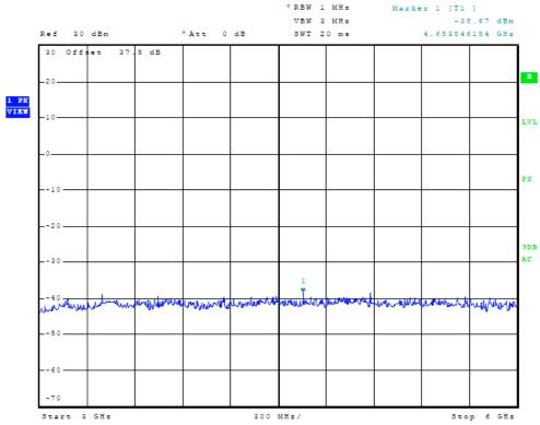
Figure 8 Spurious Emissions at Antenna Terminal (UAT 978 MHz T1)
