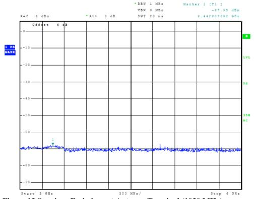
Figure 13 Spurious Emissions at Antenna Terminal (1030 MHz)
