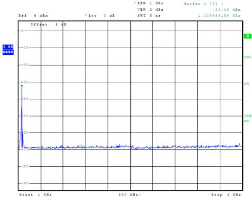
Figure 12 Spurious Emissions at Antenna Terminal (1030 MHz)
