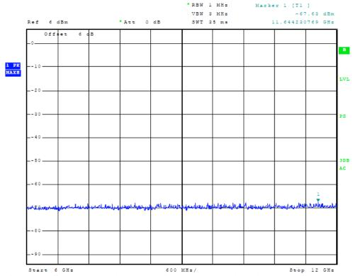
Figure 14 Spurious Emissions at Antenna Terminal (1030 MHz)
