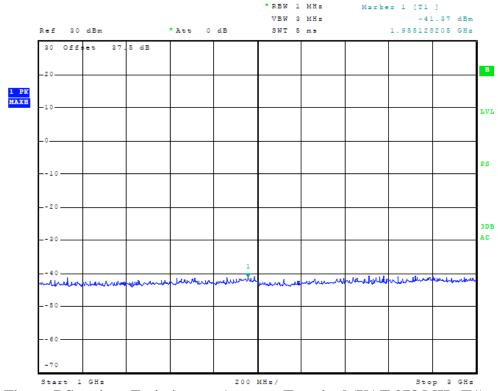
Figure 7 Spurious Emissions at Antenna Terminal (UAT 978 MHz T1)
