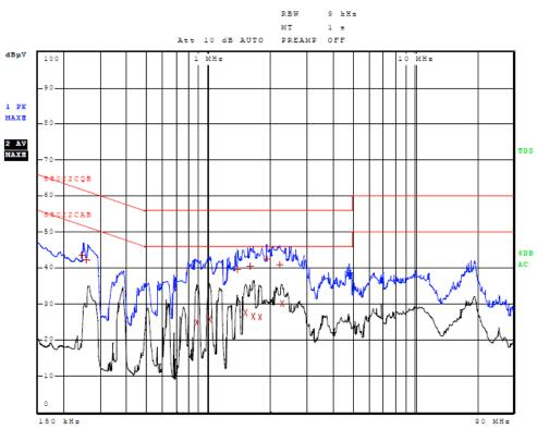
Figure Four AC Line Conducted emissions of EUT line 2 (EUT – USB -CPU AC Adapter)
