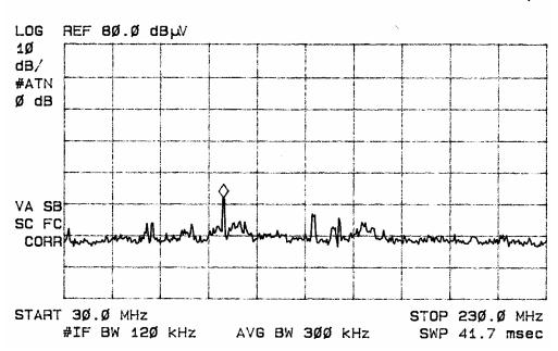
Figure three Radiated Emissions taken at 1 meter in screen room configuration #2.
