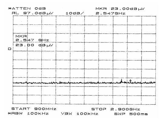
Figure five Radiated Emissions taken at 1 meter in screen room configuration #2.
