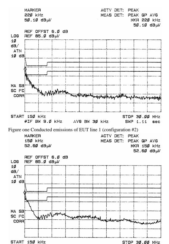
Figure two Conducted emissions of EUT line 2 (configuration #2)
