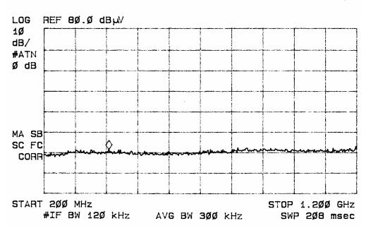
Figure four Radiated Emissions taken at 1 meter in screen room configuration #2.
