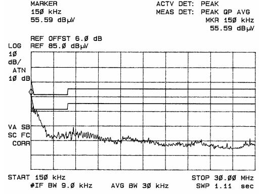
Figure four Conducted emissions of CPU and EUT line 2
