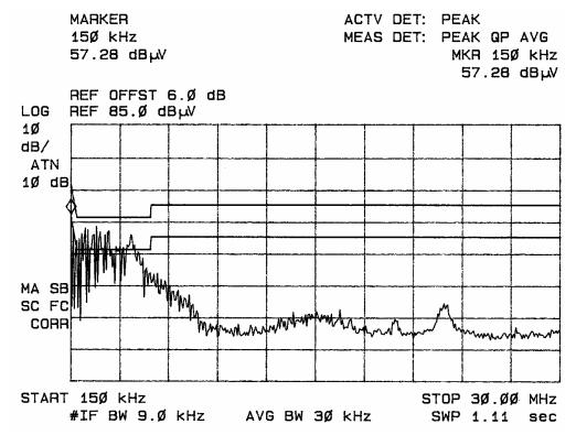
Figure one Conducted emissions of EUT line 1
