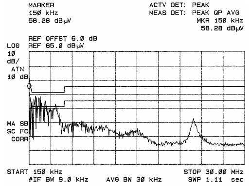
Figure two Conducted emissions of EUT line 2
