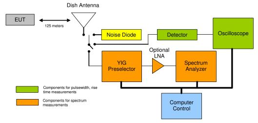
Figure 1. Measurement diagram.
