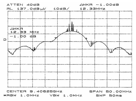
Figure three Plot of analyzer screen showing occupied bandwidth.
