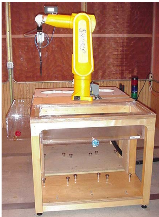
DASY4 SAR Measurement System with validation phantom
