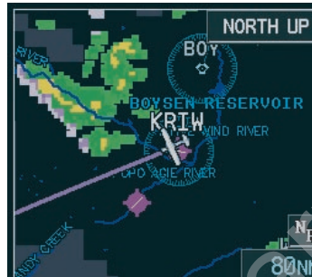
Figure 7.1.6 AUX - Trip Planning Page Map Displaying NEXRAD Weather
