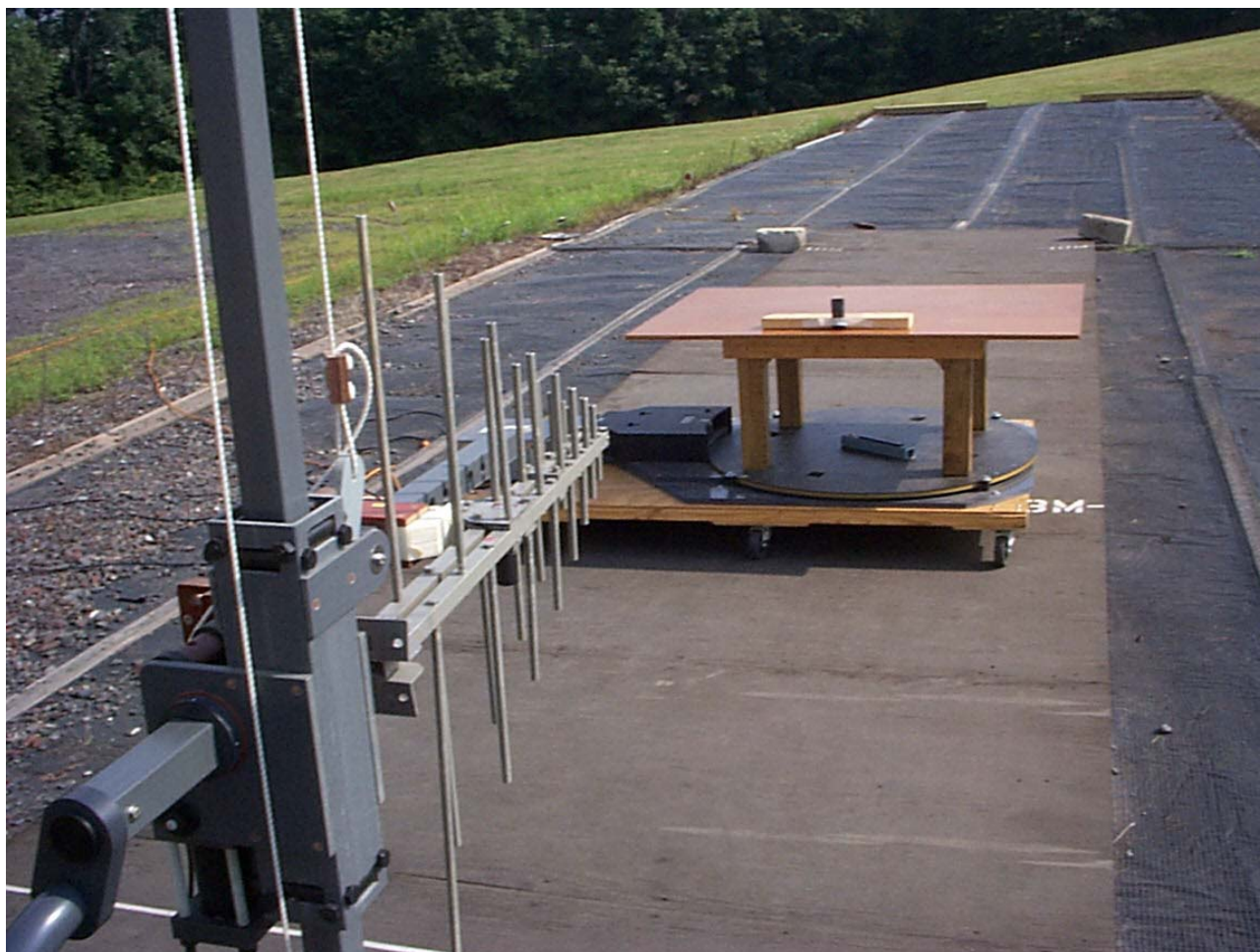
Test Range at Radiation Sciences for Substitution Method - EUT @ < 1 gig
