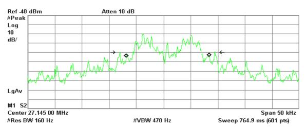
Occupied Bandwidth 15.1234 kHz Occ BW % Pwr 99.00 % x dB -20.00 dB
