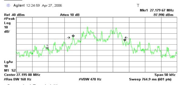
Occupied Bandwidth 15.9366 kHz Occ BW % Pwr 99.00 % x dB -20.00 dB
