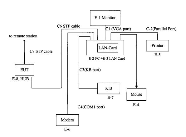
Note: E-3 LAN Card, Model <u>DFE-500TX</u>, plug-in add-on slot inside E-2 PC
