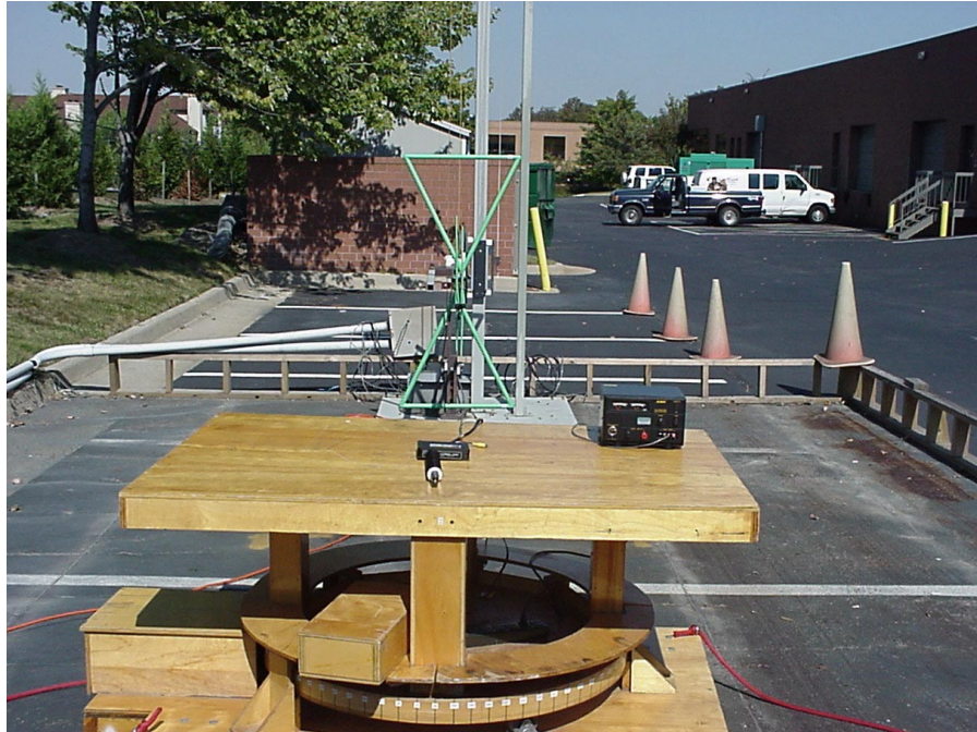
PHOTOGRAPH 1: RADIATED EMISSIONS FRONT VIEW
