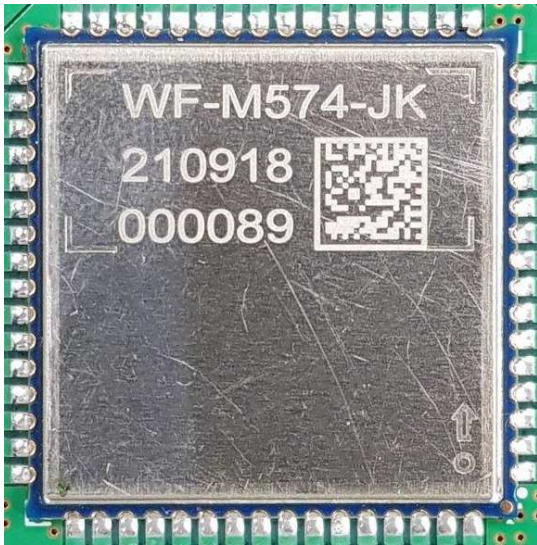
Radio Module (with Shielding case)
