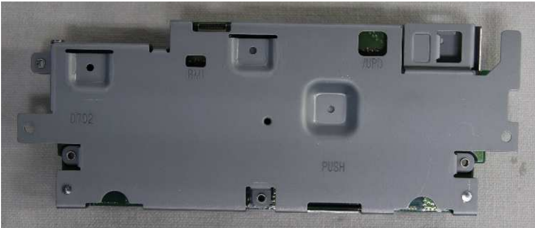
PCB with Radio module covered by shield plate
