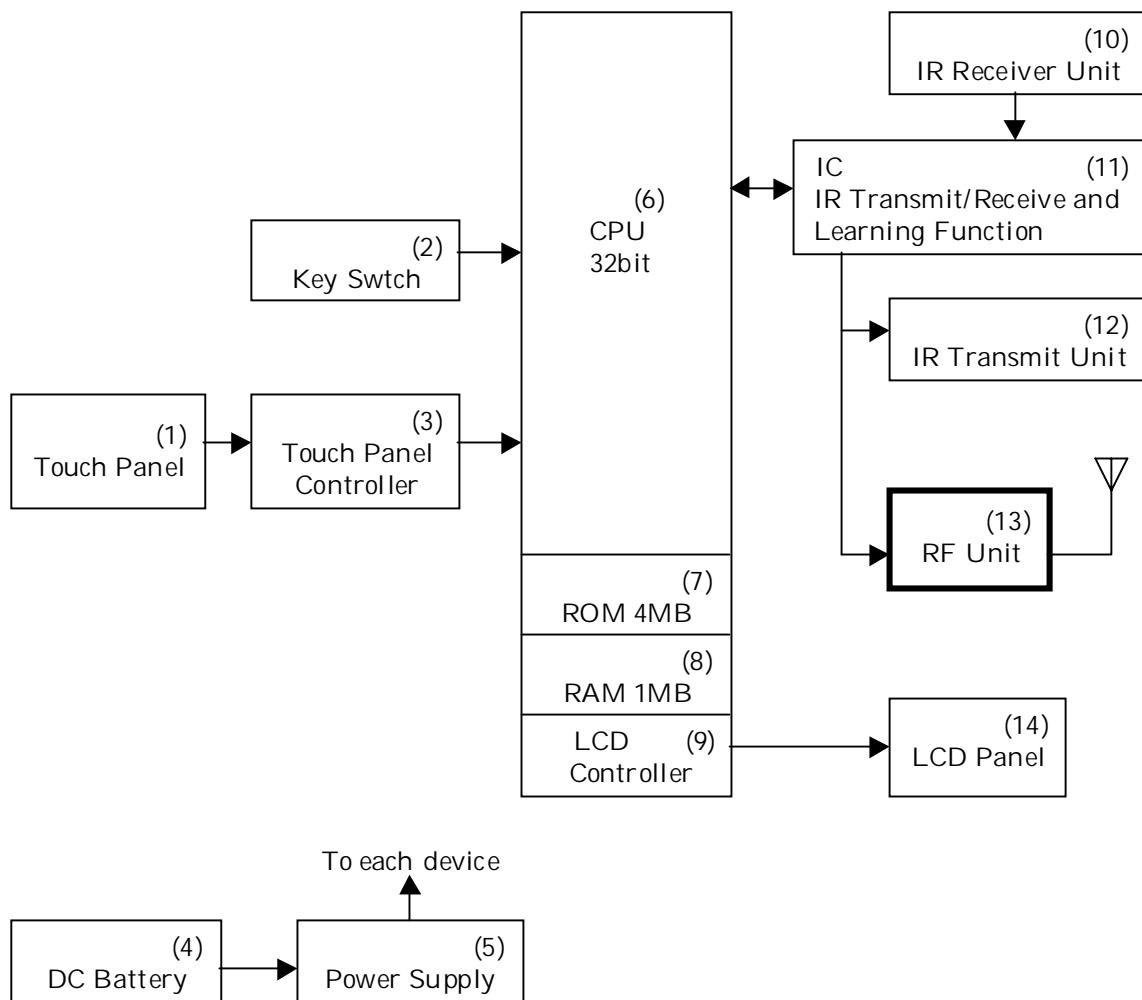
Fig.C-2 Block Diagram of RF Unit
