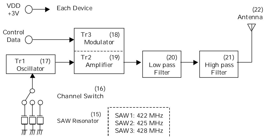
Fig.C-3 Schematic Diagram of RF Unit
