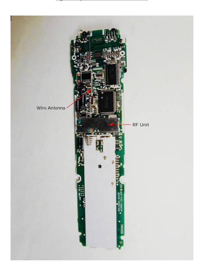
Fig.E-4 Top View of RF Unit
