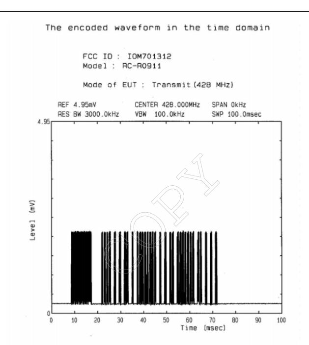
The above waveform indicates the case when field stength averaged over 100 milliseconds was maximum value. In order to obtain the peak to average factor, calculation of the period of total on-time was computed by personal computer. Results was obtaind by following. Duty cycle = (Maximum total on-time / 100 msec) x 100 = (17.3 msec / 100 msec) x 100 = 17.3 %
