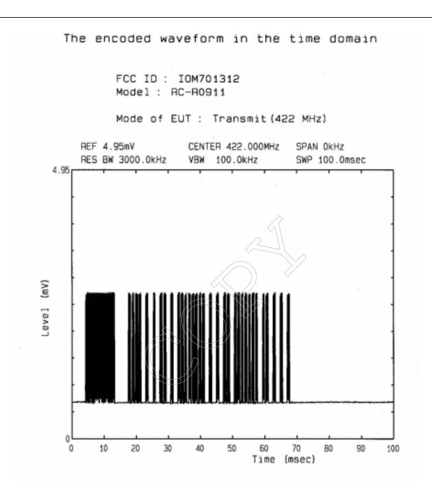
The above waveform indicates the case when field stength averaged over 100 milliseconds was maximum value. In order to obtain the peak to average factor, calculation of the period of total on-time was computed by personal computer. Results was obtaind by following. Duty cycle = (Maximum total on-time / 100 msec) x 100 = (17.3 msec / 100 msec) x 100 = 17.3 % Therefore
