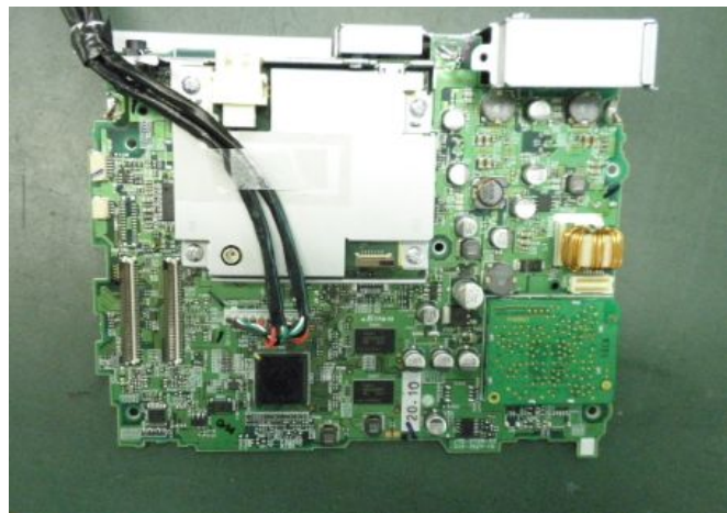
Digital Unit 3 (with shield cover)
