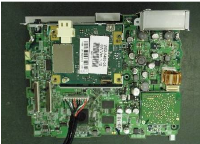
Digital Unit 2 (without shield cover)
