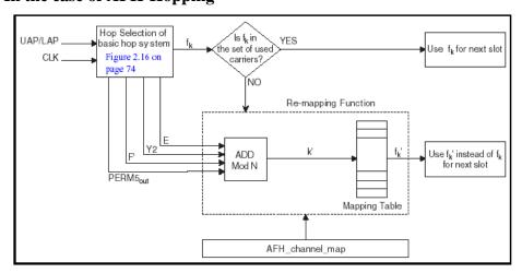
Also in the case of AFH, the fundamental sign adopt the sign head 160that is the same as the case of 79Hopping. Hopping Pattern uses the value that is worked out by dividing with the number of AFH-Channel's. Then, available Hopping becomes even as well as 79Hopping.
