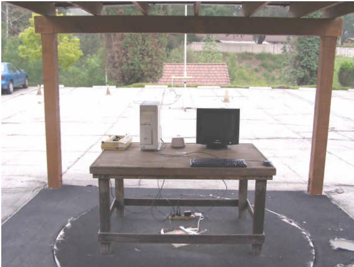
**FRONT VIEW****AVID IDENTIFICATION SYSTEMS, INC.****RF ID READER****MODEL: Power Tracker VII****FCC SUBPART B AND FCC SUBPART C – RADIATED EMISSIONS – BELOW 30 MHz****PHOTOGRAPH SHOWING THE EUT CONFIGURATION
