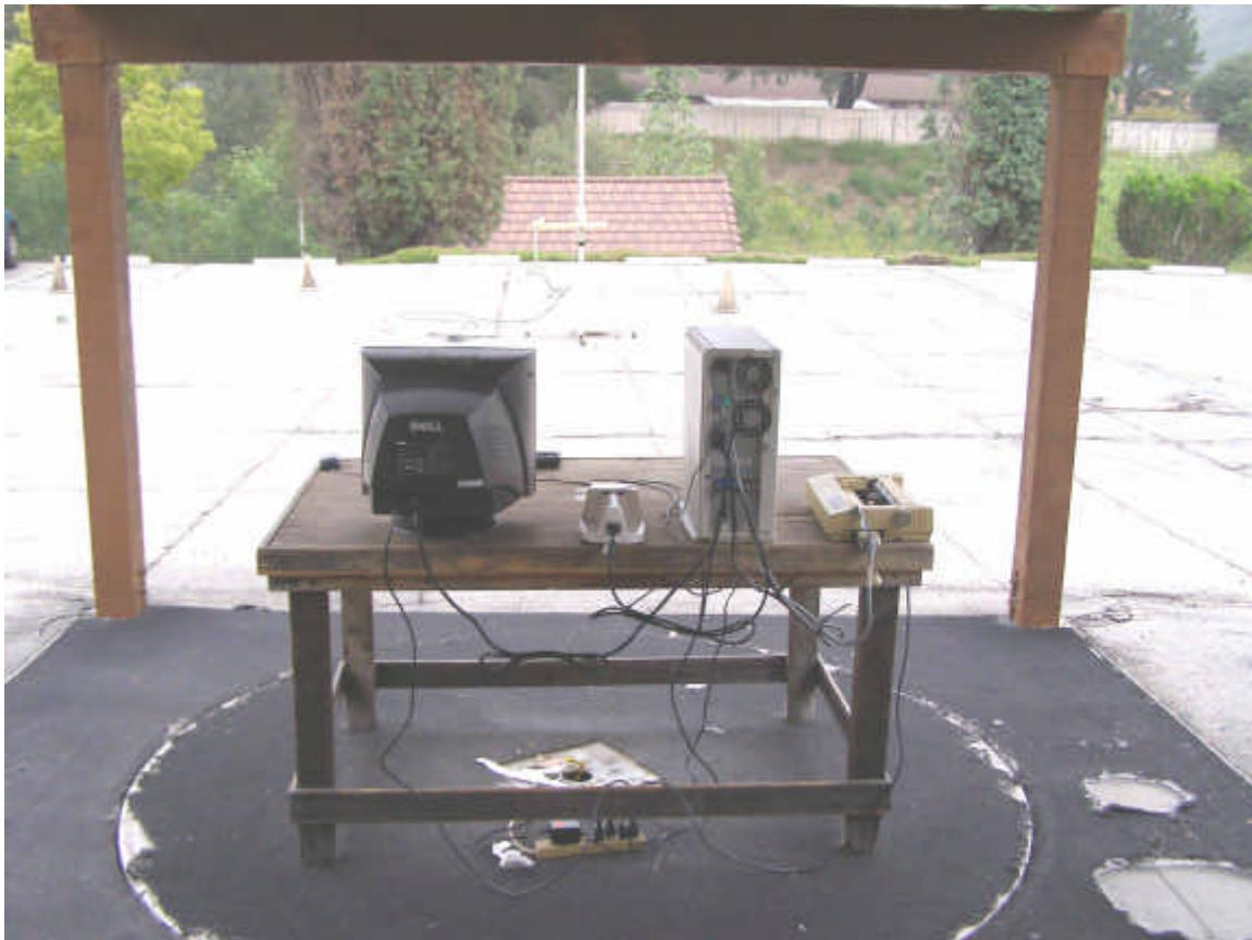
**REAR VIEW****AVID IDENTIFICATION SYSTEMS, INC.****RF ID READER****MODEL: Power Tracker VII****FCC SUBPART B AND FCC SUBPART C – RADIATED EMISSIONS – BELOW 30 MHz****PHOTOGRAPH SHOWING THE EUT CONFIGURATION
