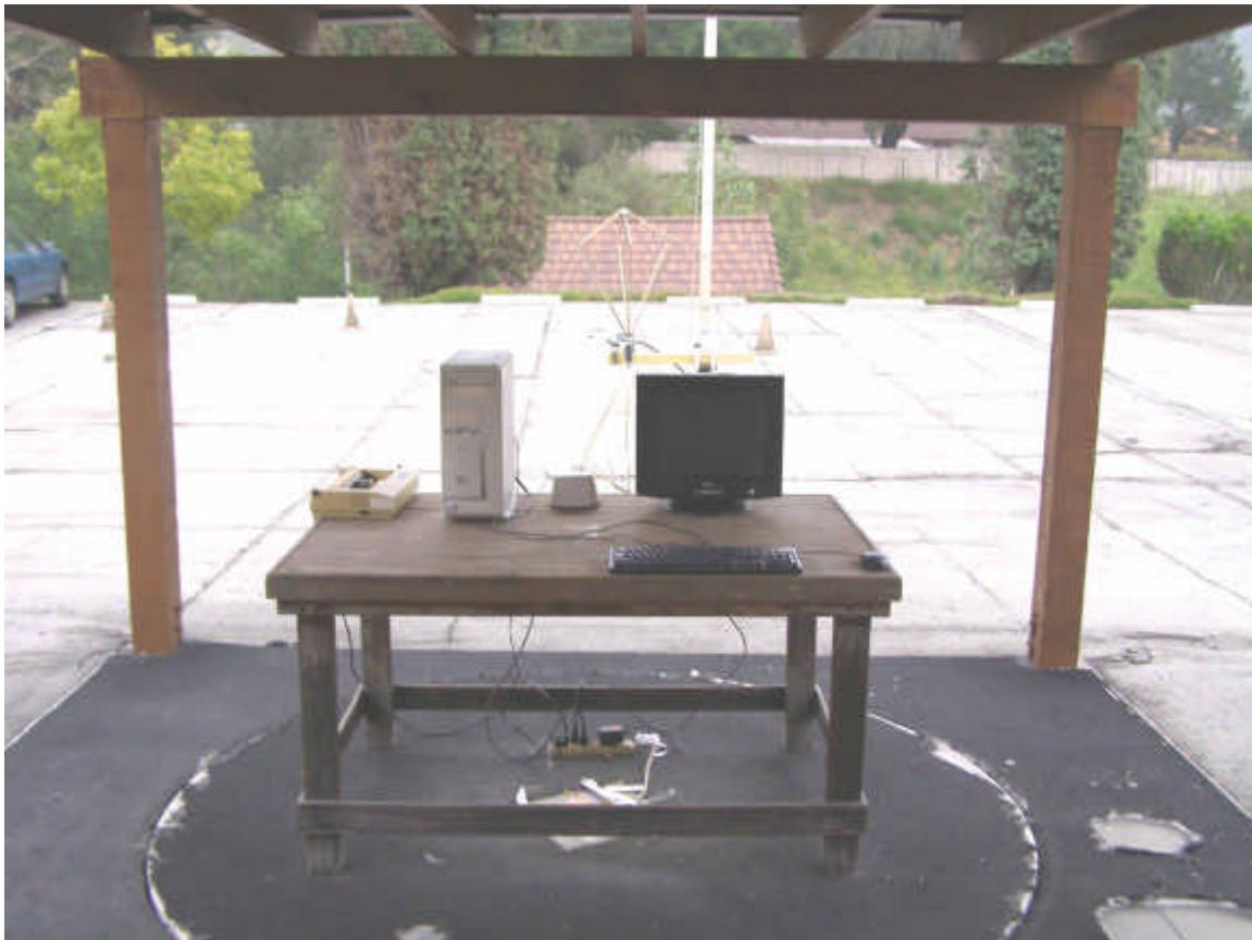
**FRONT VIEW****AVID IDENTIFICATION SYSTEMS, INC.****RF ID READER****MODEL: Power Tracker VII****FCC SUBPART B AND FCC SUBPART C – RADIATED EMISSIONS – ABOVE 30 MHz****PHOTOGRAPH SHOWING THE EUT CONFIGURATION
