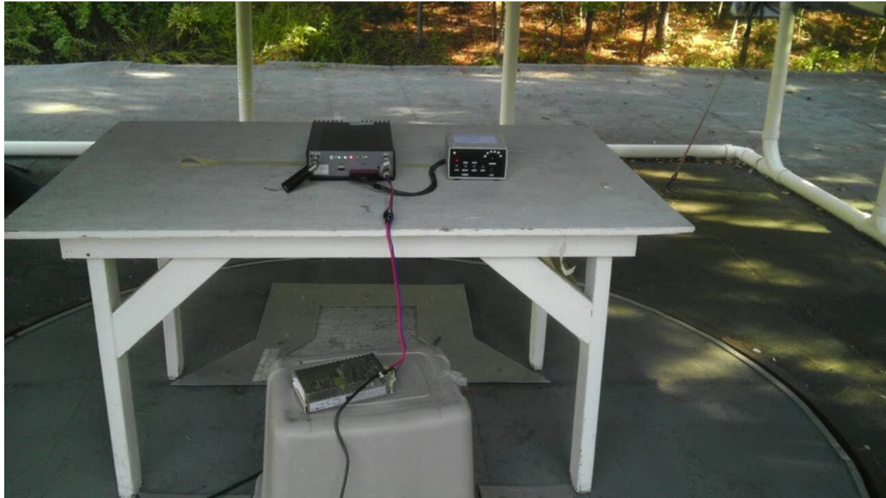
Figure 2 - Photograph of Spurious Radiation Test Setup, (Front View)
