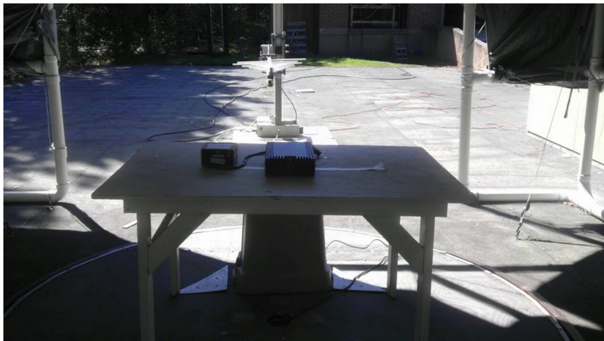
Figure 3 - Photograph of Spurious Radiation Test Setup, Rear View
