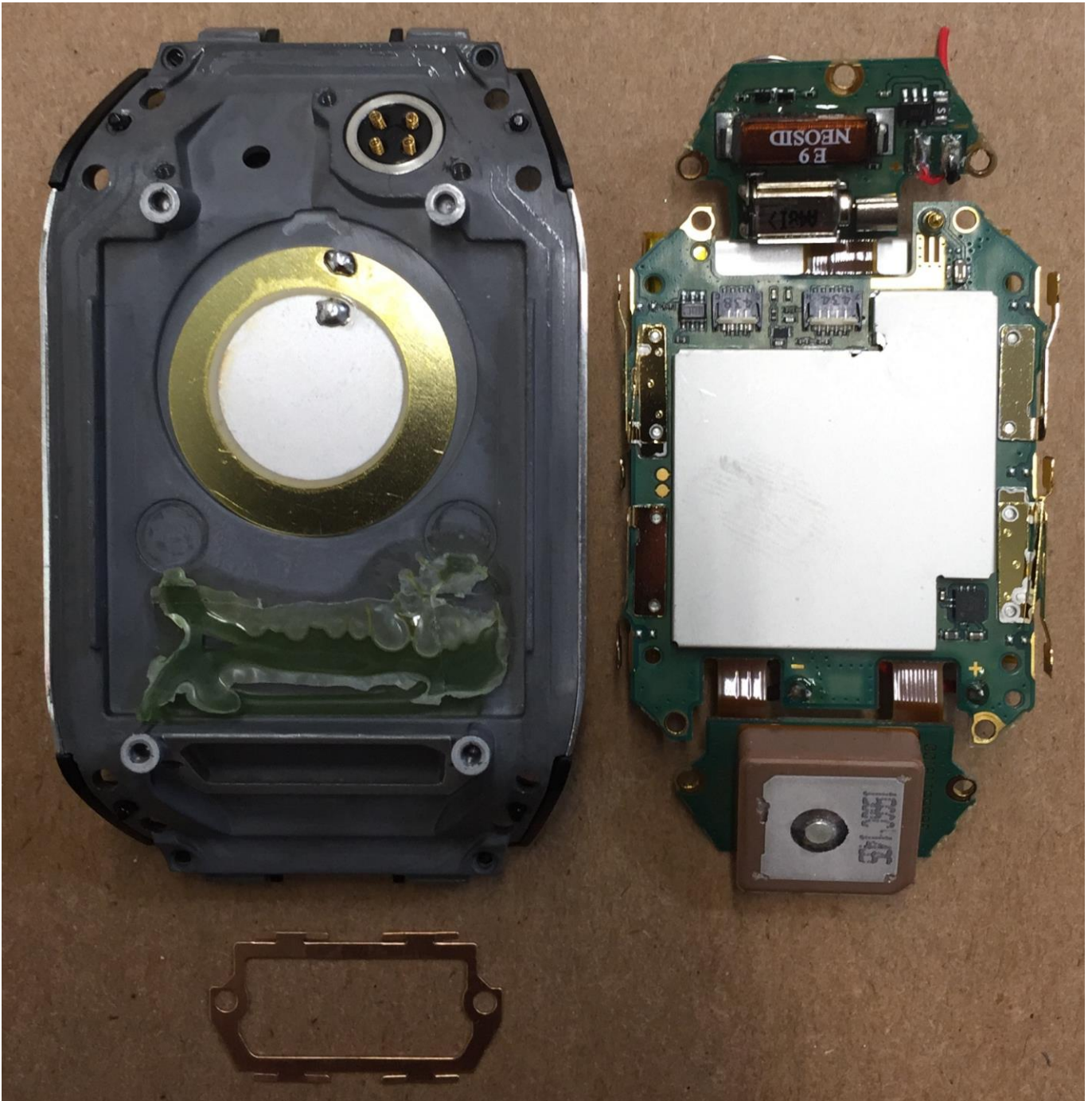
Figure 3. Electronics module detached from the back cover.
