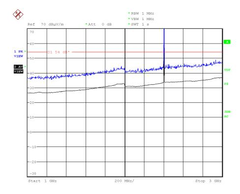
Note: The peak shown in the plot is the carrier frequency.
